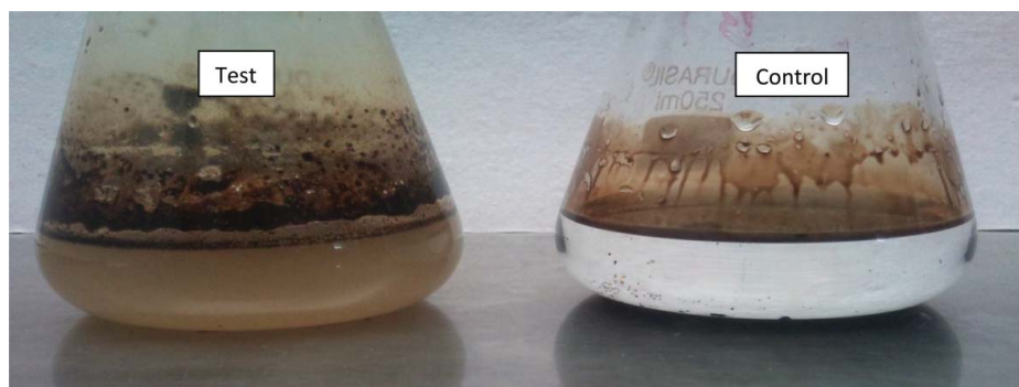
Figure 6. Dispersion of degraded crude oil due to degradation by Nocardia farcinica after incubation of 10 days at 37°C.
