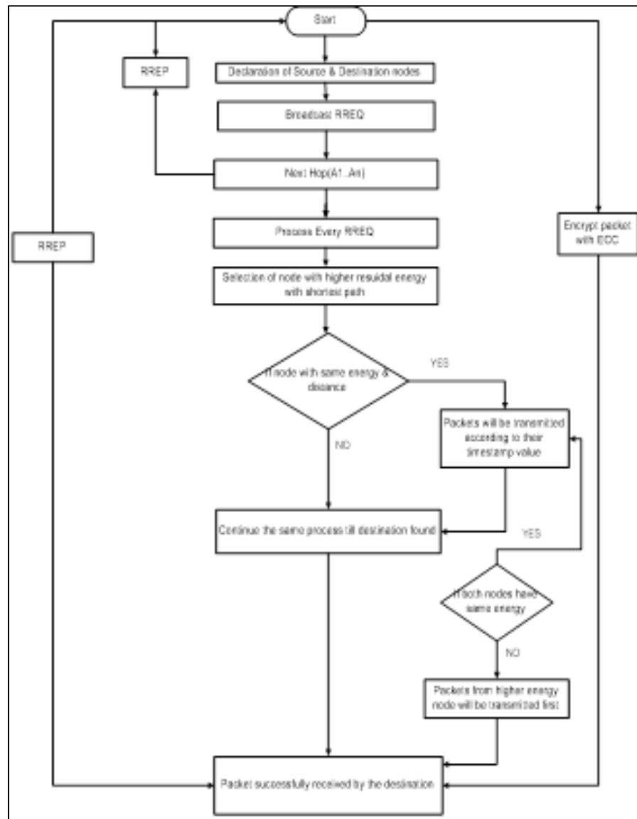
Fig. 1: Flow chart for route discovery with AOMDV protocol
