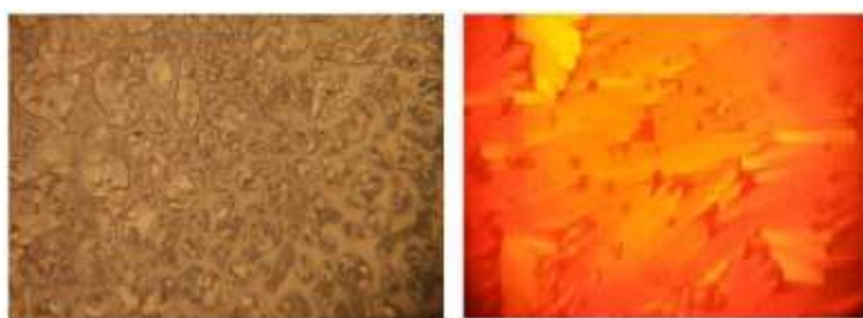
Figure 2: Microphotographs of texture observed for compound (a) Schlieren texture of Nematic mesophase on heating at 137 °C (Series I; n=7 ). (b) Focal conic texture of Sm-A mesophase at 122 °C on heating (Series I; n=7 )
