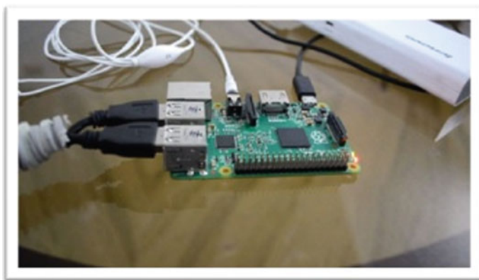
Fig. 4 Raspberry Pi 3 B+ processor board
